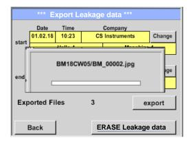
Press the "Export"- button to transfer the selected data to the USB stick In the example given, 3 measurements are exported.
