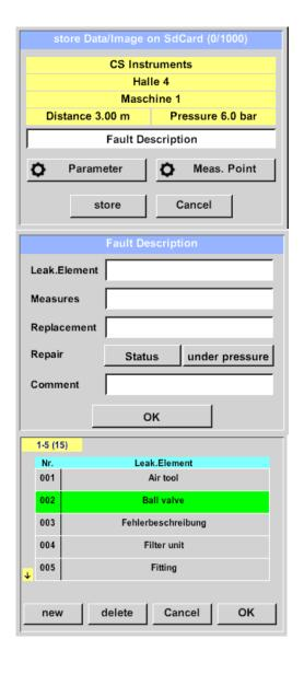
In addition to the details of the measuring point with company, building and location, it is possible to enter a fault description
