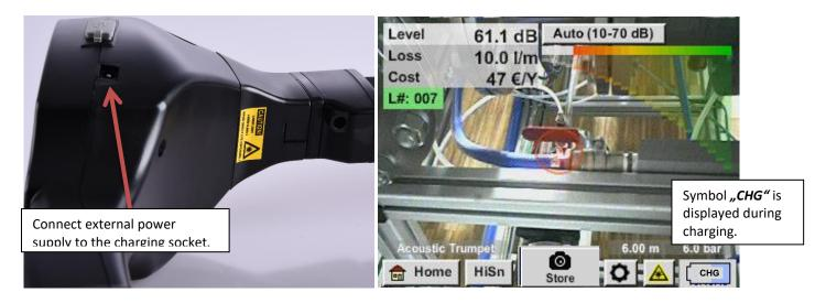
The LD 500 checks the charging status of the battery and starts the charging process automatically if necessary.
