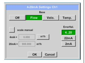
Selection of the analogue output measurement value by activating the appropriate measured value key in this example, "Flow".
