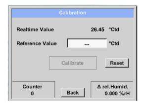
Here, a one-point adjustment can be performed.
