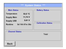
The menu item "System status" provides information about the power supply voltages and an operating hour counter.
