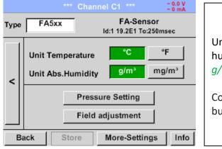
Unit selection for temperature and humidity by pressing the button  $^{\circ}C$ ,  $^{\circ}F$ ,  $g/m^3$  or  $mg/m^3$ .
