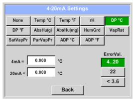
This menu allows the adjustment / assignment of the measurement value and the scaling of the analogue output.
