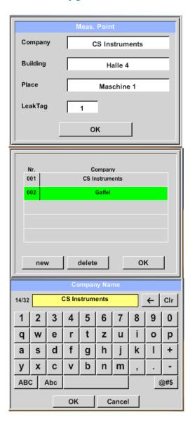
The measuring point is stored for each leakage in its journal data. These can be seen later in the leakage report in the software.
