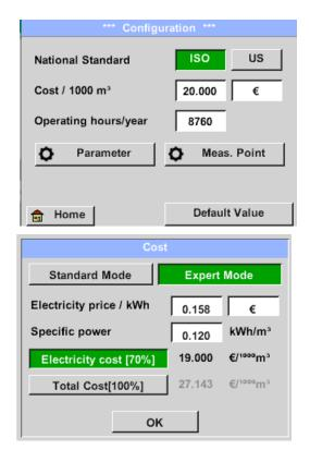
In the configuration settings the unit system can be selected and the required parameters entered, this to calculate the leakage costs per year.
