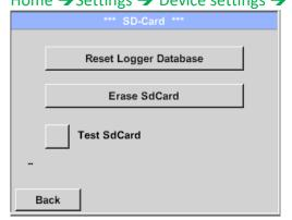
By pressing *Reset Logger Database* all actual stored data on SD-Card will be blocked for use in LD500 / LD510. Nevertheless all data are still stored and available for external use only.
