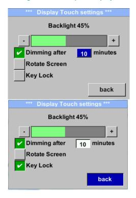
With the button "-" and with button "+" it is possible to adjust the backlight / display brightness. The actual / adjusted backlight brightness is showed in the graph "Backlight."
