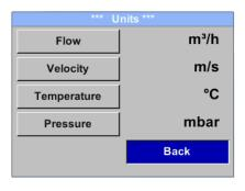
To make changes to the unit for the respective measurement value, first select by pressing ">" the field of the "measurement value" and activate "it with "OK".
