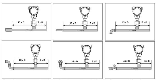
The values represent the min.lenghts. In case the min. inlet / outlet runs could not be ensured, it must be expected to get increased or significant deviations of the measurement values.
