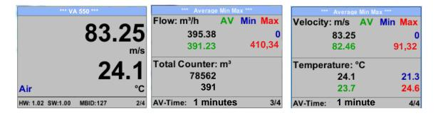
AV-Time ( Period for average value calculation) could be changed under *Sensor Setup.-Advanced– AV-Time*
