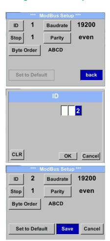
For changes, e.g. the sensor ID, select with key "△" the field "ID" and then pressing "OK".
