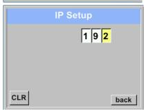
For manual (static) IP, the "IP Address", "Subnet" and "Gateway" selection keys must be selected and activated with "OK".
