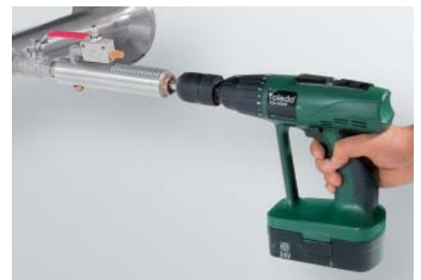
• Drilling under pressure
