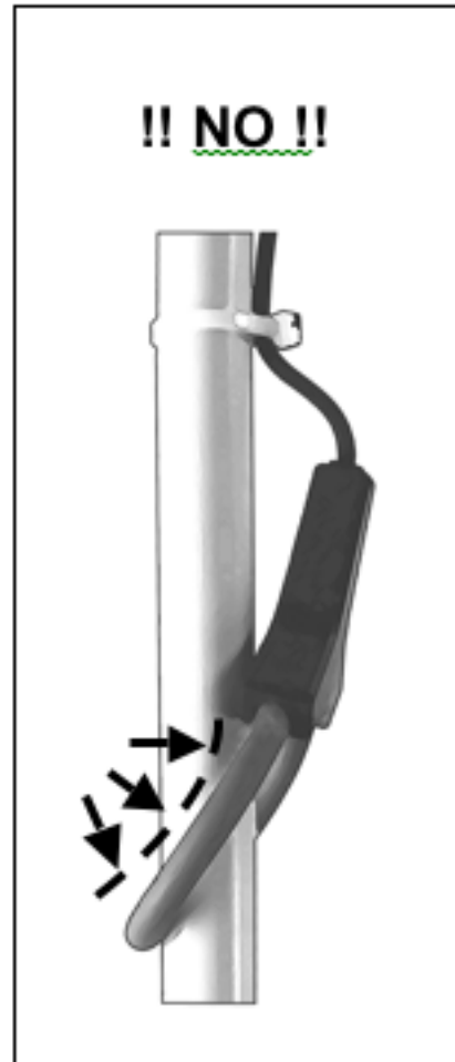
Fig. 4: take care to avoid mechanical distortion
