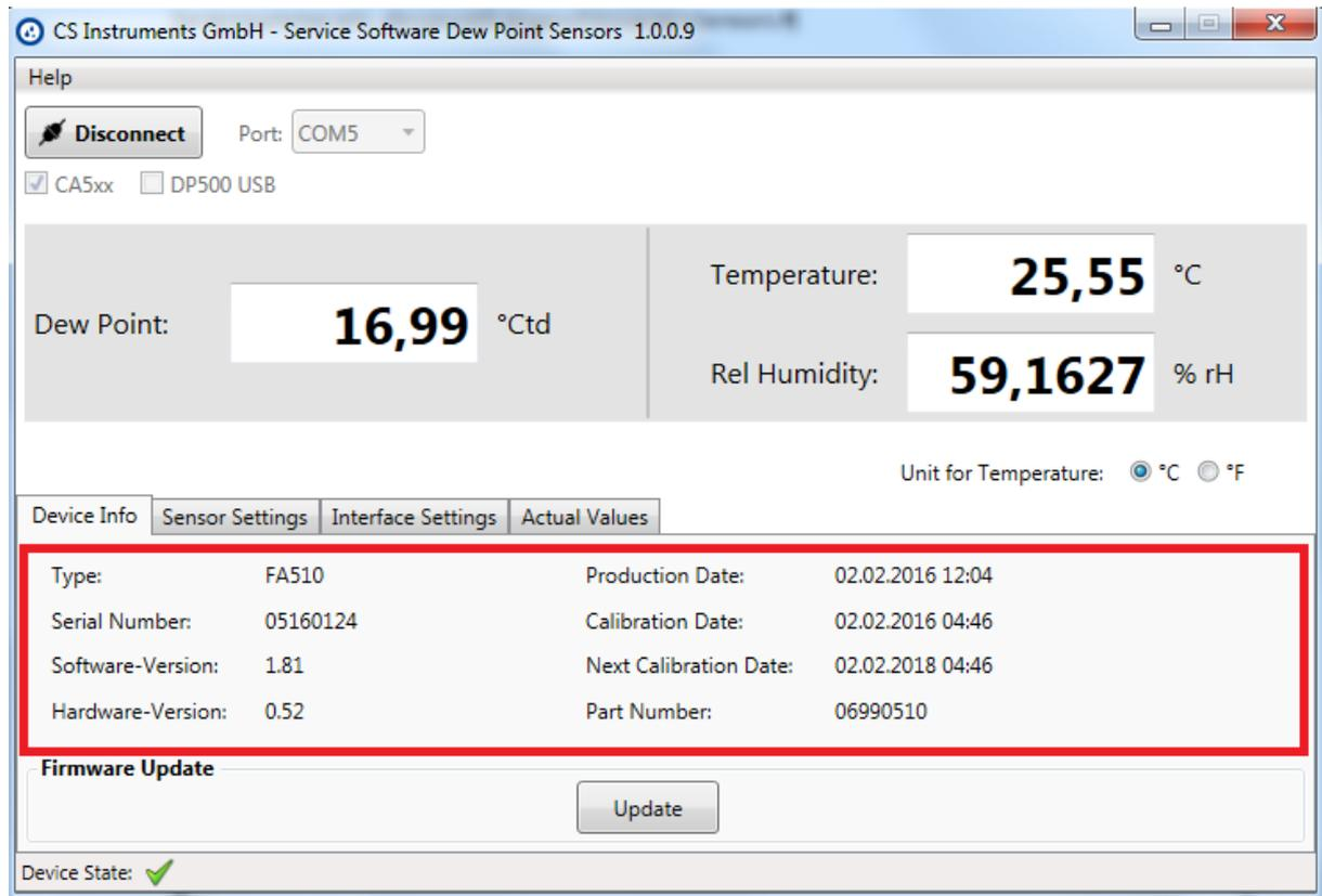
The tab "Device Info" shows an overview about different specific information. For example: The serial number of the connected dew point sensor, Production date etc.
