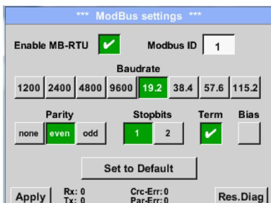
By communication via Modbus TCP the *Modbus Id* have to be set only and confirmed by pressing *Apply* button
