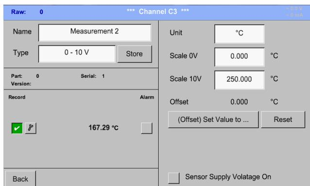
Please see the scale of the sensor (here for example **Type 0 - 10V** corresponds to 0 - 250 °C) from the data sheet of the connected sensor.
