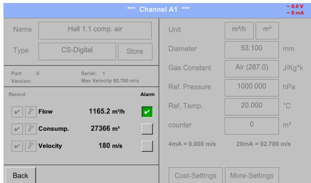
Like in *Main → Real time values*, individual channels can be selected here, to detect which and how much the value has exceeded or below the alarm range.
