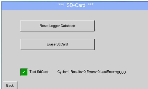
By pressing *Reset Logger Database* all actual stored data on SD-Card will be blocked for use in DS500. Nevertheless all data are still stored and available for external use only.
