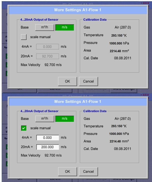
In *More-Settings*, you can define whether the 4 - 20 mA analogue output of the sensor based on the flow rate or velocity.
