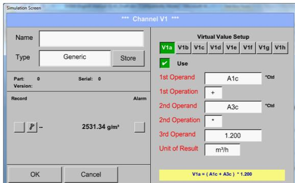
The *Resolution* of the decimal places, the *Short Name* and *Value Name* are found under the **Tool button**
