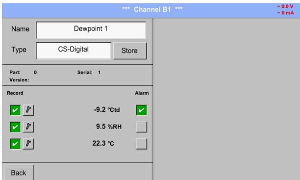
The DS 500 detects, if the connected sensor is a flow or dew point sensor of **CS Instruments** and set the *CS-Digital* subtype automatically correct.
