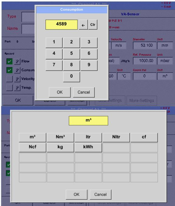
The sensor allows taking over a starting counter value. Inserting the value by entering the "Count. Val." text field.
