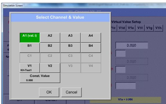
By pressing a button either for HW-, virtual channel or const. Value e.g. *A1* a list of all available measurement channels or measurement values will appear.
