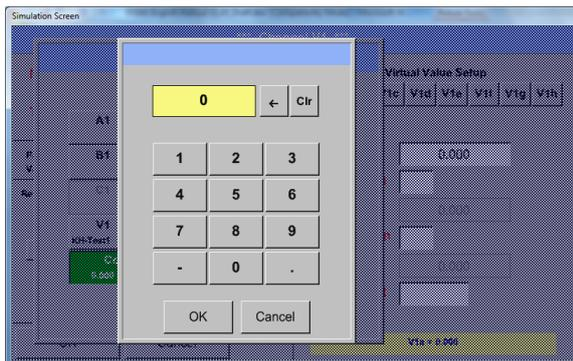
Pressing the button **const. Value** requests the input of the **const. Value** into the text field.
