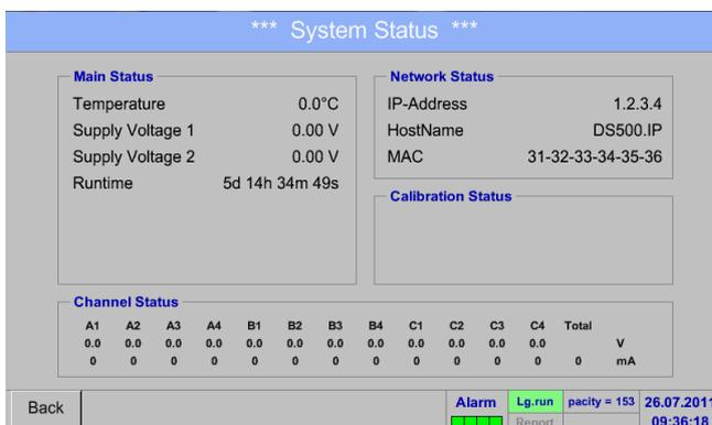
The function **System Status** offers an overview, fitting voltages and currents on the individual and the entire channels, as well as the power supply of the power supply units.
