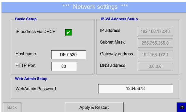
Here you can set up and made a connection, with or without *DHCP*, to a computer.
