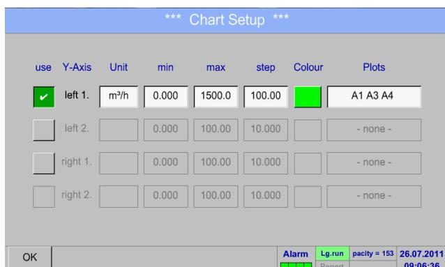
6. The *Plots* description field shows on what channel the measured data were recorded and there can be seen how much recordings on one y-axis are represented.
