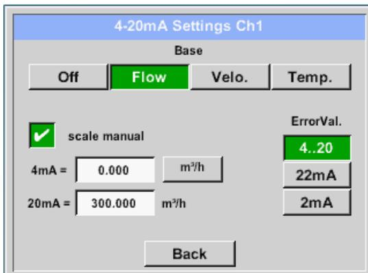
This menu allows the adjustment / assignment of the measurement value and the scaling of the analogue output by pressing the "4-20mA Ch1" button.
