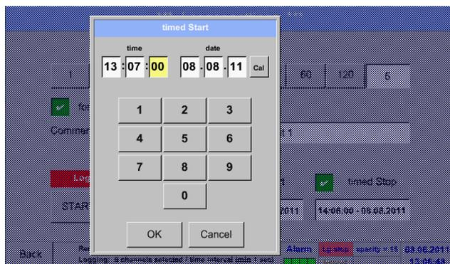
After pushing the *date/time description field* a window will appear where the yellow marked area of the time or date can always be set and changed.
