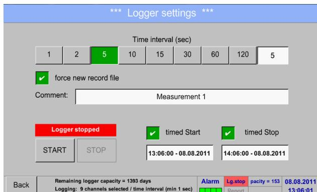
By pushing the *timed Stop* button and then the date/time description field below, the date and the stop time can be set for a data logger recording.
