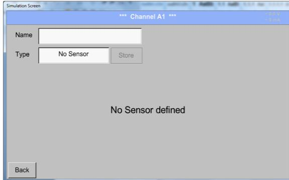
By pushing the description field *Type No Sensor* the list of sensor types appears (see next step).
