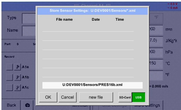
Using the buttons *SD card* or *USB*, the storage location will be determined.
