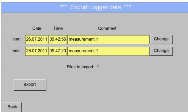
Use the *Change* buttons to adjust a period between *start* and *end*. Stored measurement data in this period are exported.
