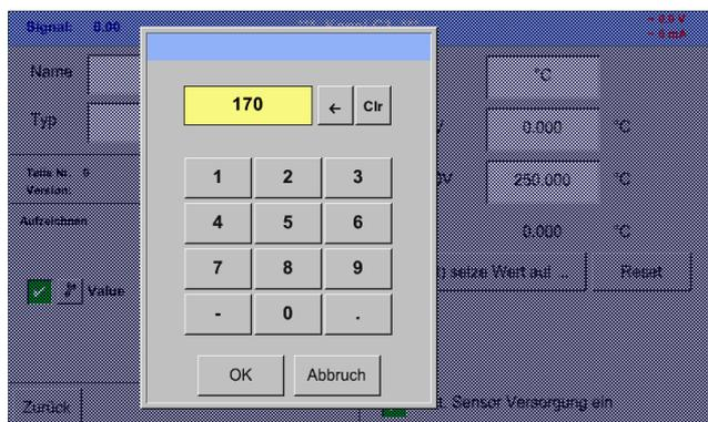
With *Set-Value to-(Offset)* it is possible to set the measurement data to specific value.
