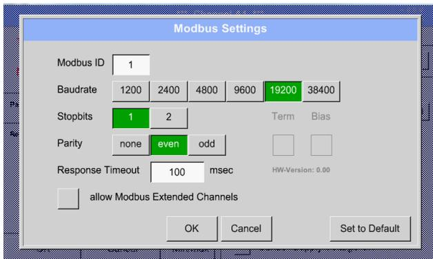
Here are the corresponding values for *Modbus ID*, valid values are 1-247, (e.g. here Modbus ID = 1.), the serial communication settings *baud rate*, *stop bit*, *parity and timeout* to define. Is the DS500 connected at the end of the bus the termination and BIAS to be enable by pressing buttons Term and Bias.
