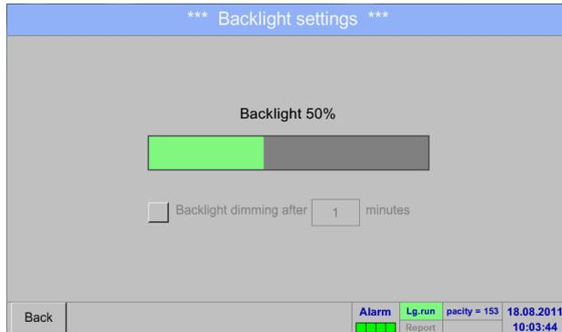
Here you adjust the desired *Backlight* (15-100%) of the display directly.
