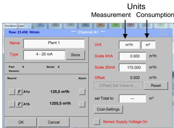
Selection of the units by pushing the text fields for the corresponding measurement and consumption units.
