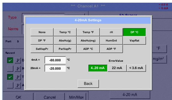
This menu allows the adjustment / assignment of the measurement value and the scaling of the analogue output.
