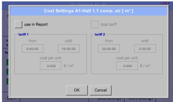
In the *Sensor settings* for the *Type CS-Digital* and *Pulse* you can enter the costs per unit in the *Cost Settings*.
