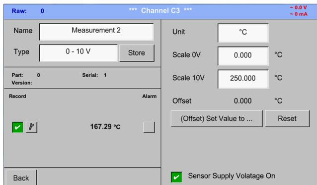
The *Sensor Supply Voltage* is switched **On**, if it's required by the sensor type, otherwise off (no green hook).
