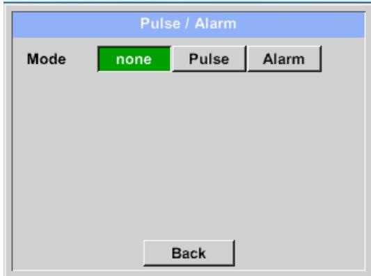
The pulse output of the VA 5xx could be set functionally as pulse output or alarm output.
