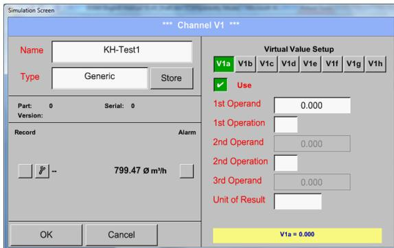
Every virtual value has to be activated by selecting the respective *Value-Button* e.g. *V1a* and pushing of the *Use Button*.
