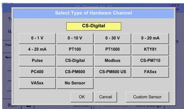
Now the **Type CS-Digital** is selected for the VA/FA 400 series and confirmed by pressing the **OK** button.
