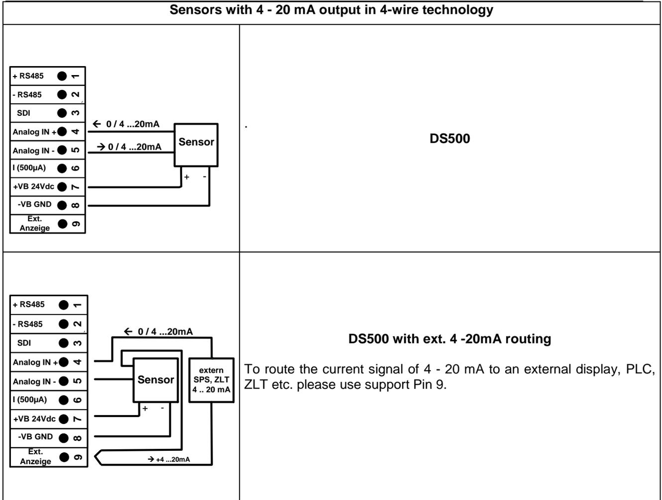
11.5 Three- and four-wire power supply 0 - 1/10/30 VDC
