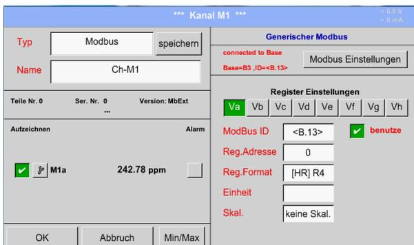
The *Modbus ID* is at initial activation taken over as a copy of the *Modbus settings* of the base channel (marking: value in <>), but it can be overridden.
