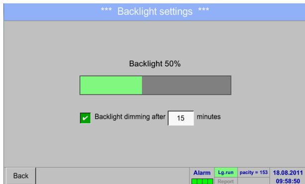
With the help of the *Backlight dimming after* button, after a definable time interval (here after 15 minutes), the *Backlight* can be reduced to the minimum.
