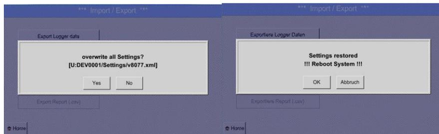
After confirmation with OK it is asked again if settings should be overwritten, by confirming this once more the new System Settings are loaded and a reboot is required.
