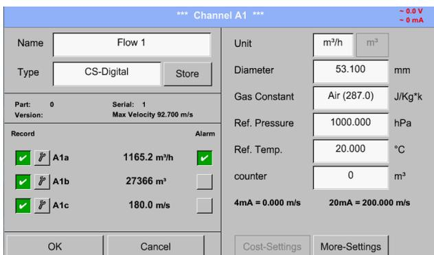
The DS 500 detects, if the connected sensor is a flow or dew point sensor of **CS Instruments** and set the **CS-Digital** subtype automatically correct.
