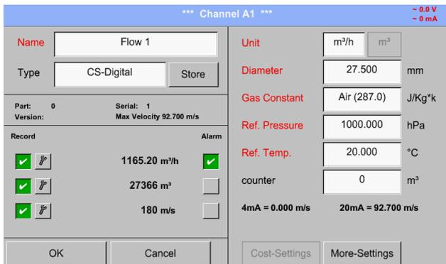
The red labeled description fields indicates that different values, such as the *Diameter* and the *Name*, have been changed or added.
