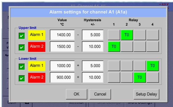
E.g. set the *Alarm 1* to relay 2 and relay 4 and the *Alarm 2* to relay 1 and relay 3.
