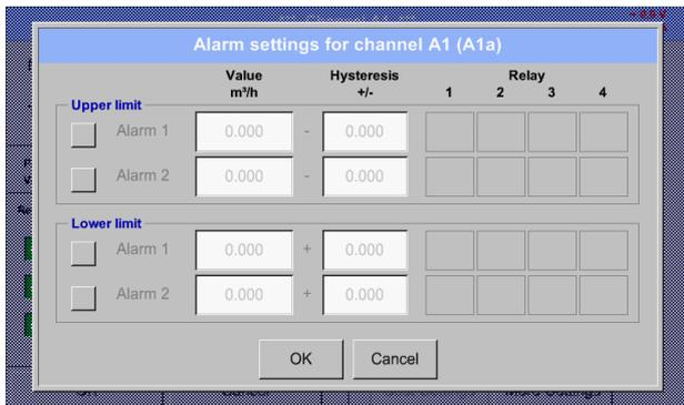
In the alarm settings, an *Alarm 1* and *Alarm 2* incl. *Hysteresis* can be entered for each channel.
