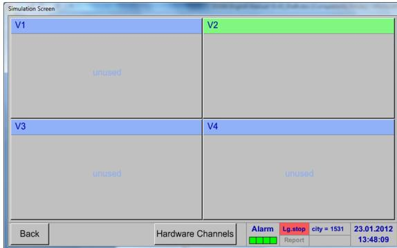
After pushing the button „*Virtual Channels*“ in the Sensor Settings menu an overview with the 4 available “*Virtual Channels*” is displayed.
