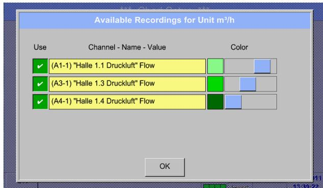
5. Several recordings with the same unit can be represented in one y-axis, with the help of various colour intensities.
