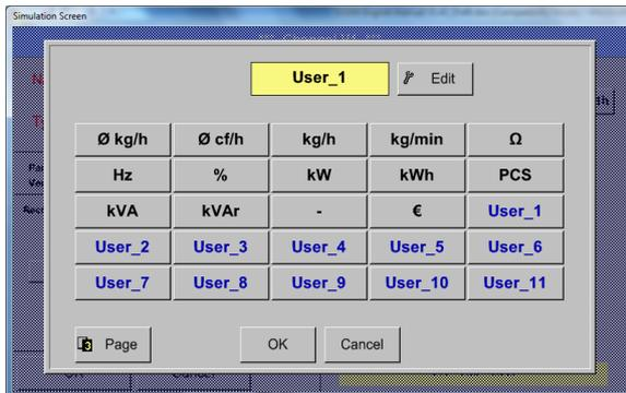
By pressing the button *Edit* you enter the menu for inserting the new Unit.
