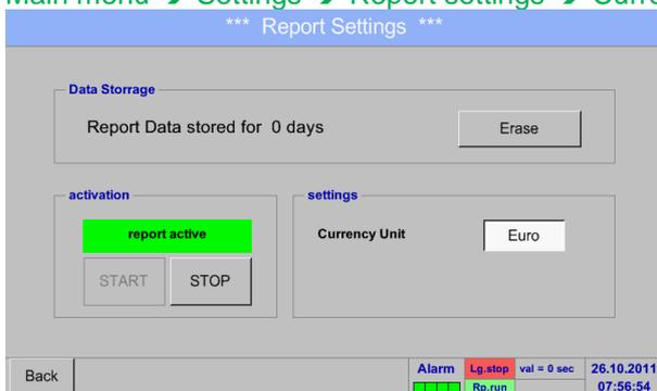
By pushing of the *Currency Unit* description field, a currency may be entered, which is applied to the **Consumption report** and the **cost settings**.
