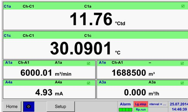
The view *Real time values* allows displaying of 1 to 10 free definable measurement values.
