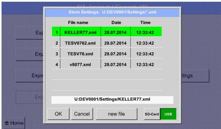
With Export system settings, all existing sensor settings can be exported to a USB stick or to the internal SD card. It stores all sensor settings including recording-, alarm-, graphics-, value- and name definitions. Storing location could be selected using the buttons *SD card* or *USB*.
