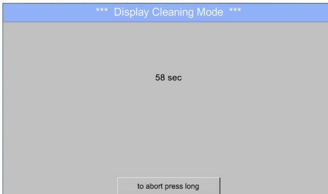
This function can be used for cleaning the touch panel during running measurements.
