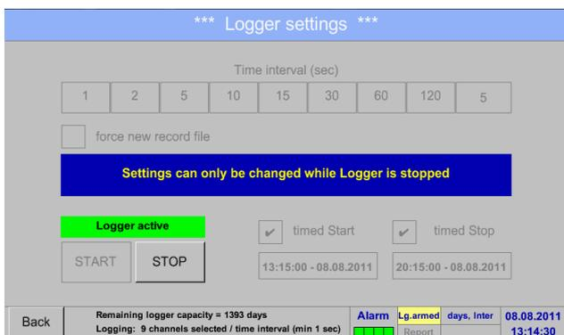
After the start and stop time activation and the created settings, the *Start* button will be pushed and the data logger is started.
