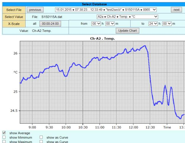
**Select File :** In this drop down field a measurement data file could be selected. With buttons *previous* & *next* could be switched between the files
