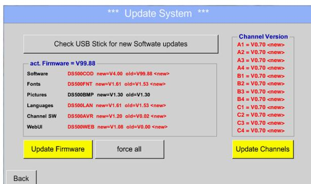
Is the DS 500 properly connected to the USB drive and there are new versions of the individual software parts available, then they are in red font and <new> marked.
