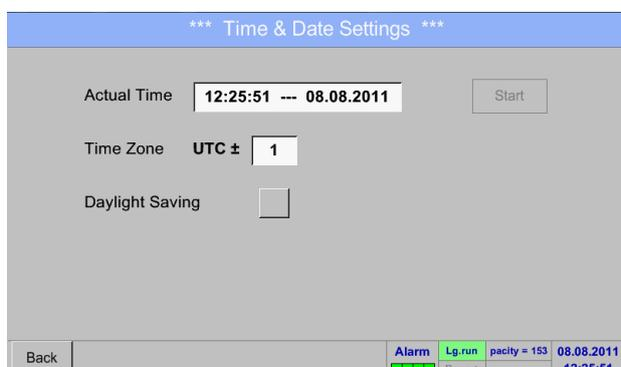
By pushing the *Time Zone* description field and enter the correct *UTC*, you can set the correct time all over the world.
