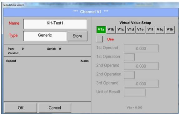
By pushing the Text field *Name* a Sensor name could be inserted.
