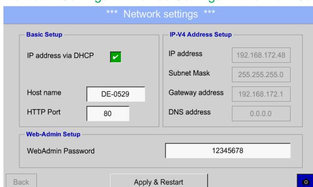
In the text description field *WebAdmin Password* could the password be set up. The password length is  $\geq 6$  characters.
