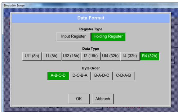
With the buttons *Input Register* and *Holding Register* the corresponding Modbus-register type will be selected. The number format and transmission order of each value needs to be defined by *Data Type* and *Byte Order*. Both have to be applied in correct combination.
