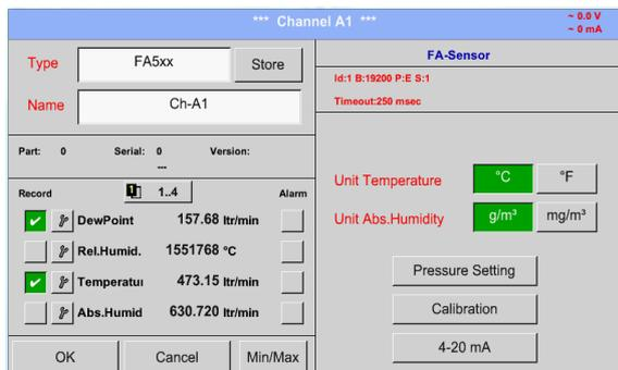
Unit selection for temperature and humidity by pressing the button °C, °F, g/m³ or mg/m³.
