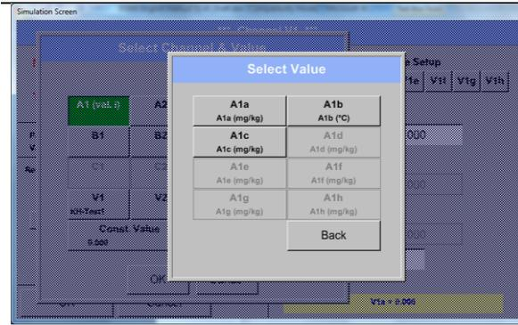
Pressing the respective channel button e.g. **A1b** will select the measurement channel
