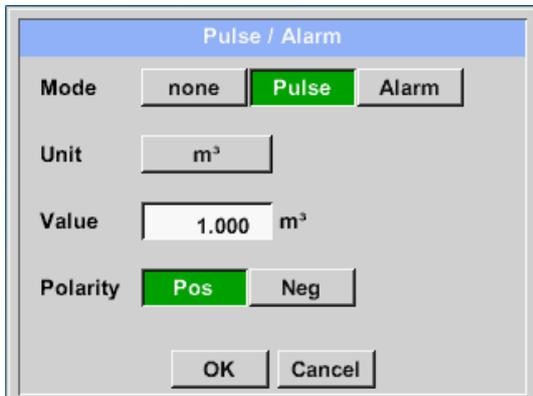
To set up the pulse first the unit and the measurement value have to be defined.
