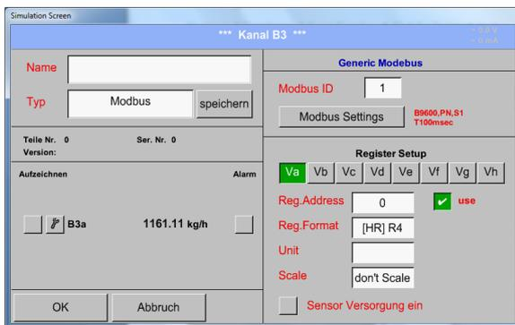
The measurement values are kept in the registers of the sensor and can be addressed via Modbus and read by the DS500. This requires to set the desired register addresses in the DS500. Entering the register / data address needs to be done in decimal with range 0-65535.
