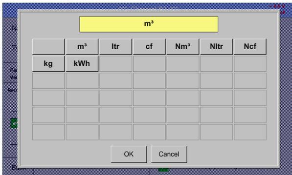
By *Unit Pulse* you can choose between a flow volume or a power consumption unit.
