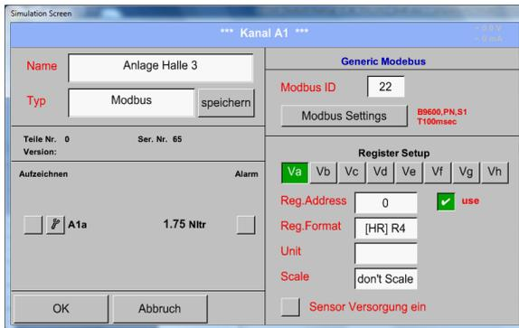
Please insert here the specified *Modbus ID* of the sensor, allowed values are 1 -247, (e.g. here *Modbus ID = 22*)
