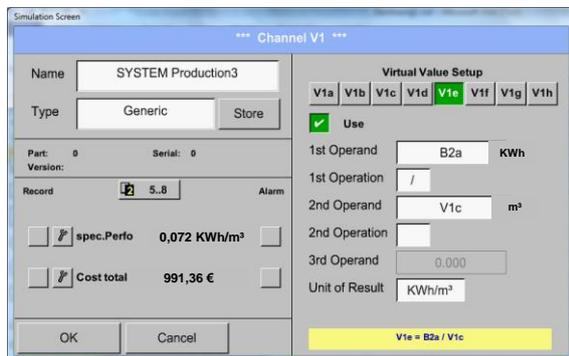
Calculation of the **specific Perfor.** Is done in **V1e** with **V1e = B2 / V1c**
