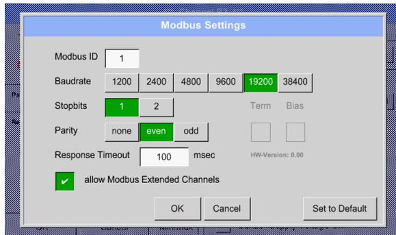
After activation of „*allow Extended Modbus Channels*“ there are 4 additional Modbus channels each with 8 values available.
