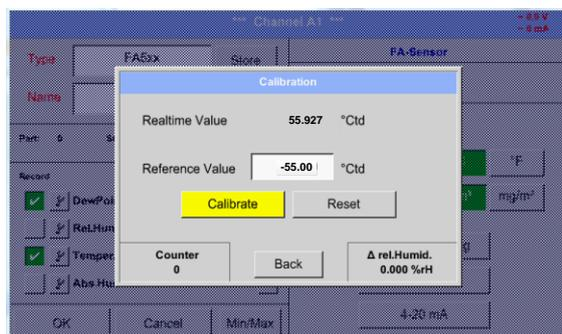
Here, a one-point calibration can be performed.
