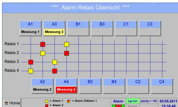
In the Alarm overview, you can immediately see whether there is an *alarm 1* or *alarm 2*. You can see also in other menu items: *Main → Real time values* and *Main → Settings → Sensor settings*. The channel name will appear yellow invers (*alarm 1*) or inverse red (*alarm 2*). In addition, you can see which relay had been set for the channel as the *alarm 1* or *alarm 2*. This is indicated by the yellow and red or red/yellow squares on the intersections between measuring channel and relay.
