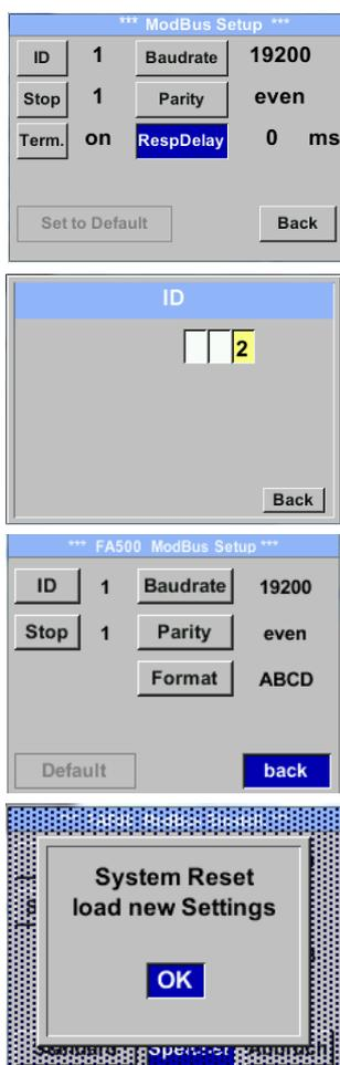
For changes, e.g. the sensor ID, first select by pressing key „ $\Delta$ “ the field “**ID**” and then key “**OK**”.
