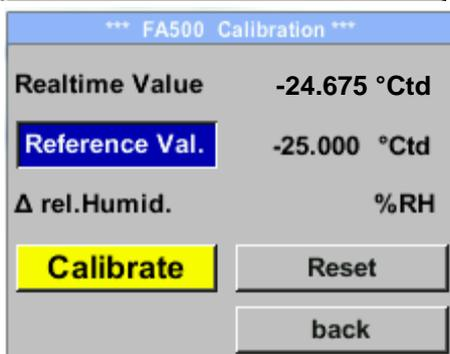
Here, a one-point calibration can be performed
