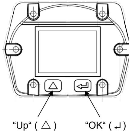
The operation of the FA 500 is done by the two capacitive key buttons Up ( $\Delta$ ) and Enter ( $\leftarrow$ )
