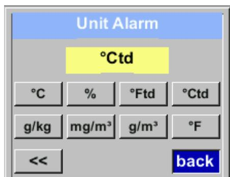
To select a measurement value, a corresponding / appropriate unit needs to be defined. Select „Unit“ with „ $\Delta$ “ and open the menu with „OK“. Select required unit with „ $\Delta$ “ and takeover it by pressing „OK“.
