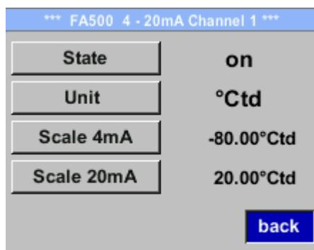
The 4-20 mA Analogue output of the Sensor FA 500 can be individually adjusted.
