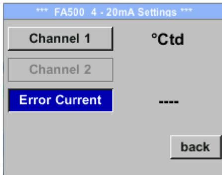
This determines what is output in case of an error at the analog output.
