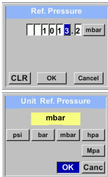
In order to change, e.g. the unit, first select by pressing key „ $\Delta$ “ the field “Units” and then key “**OK**”.
