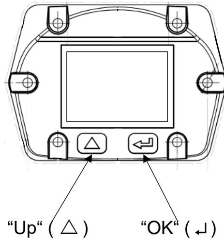
The operation of the VA 500 is done by the two capacitive key buttons Up ( $\triangle$ ) und Enter ( $\leftarrow$ )
