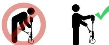
**Attention:** Alignment of the sensor must not be modified when tightening the connection thread and adapter sleeve. In this case, please check the immersion depth and alignment again and correct it if necessary. The angular deviation should not be greater than  $\pm 2^\circ$  in relation to ideal position as otherwise the measuring accuracy will decrease.
