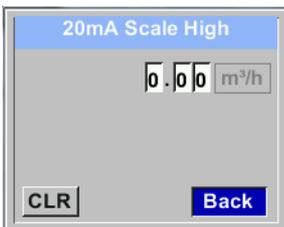
The scaling of the 4-20mA channel can be done automatically "Auto Range = on" or manual "AutoRange = off" .
