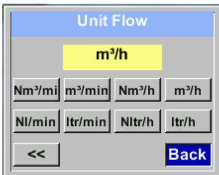
To the selected measurement value a corresponding / appropriate unit needs to be defined. Select „Unit“ with „ $\Delta$ “ and open menu with „OK“.
