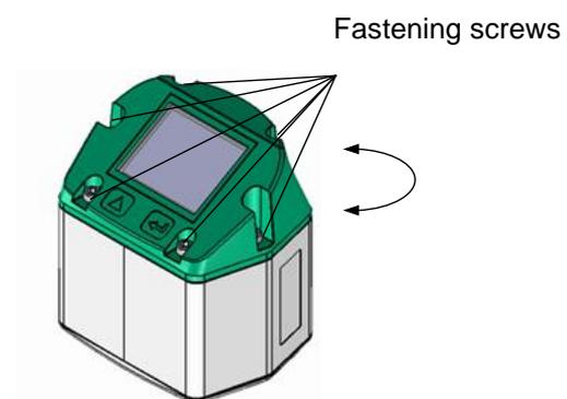
The Position of the Display head is twistable by 180 e.g. in case of reverse flow direction.
