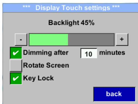
With the button „-“ and with button „+“ it is possible to adjust the backlight / display brightness. The actual / adjusted backlight brightness is shown in the graph „**Backlight.**“
