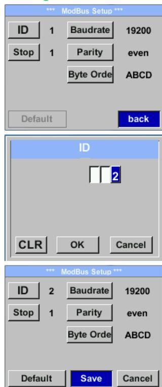
For changes, e.g. the sensor ID, first select by pressing key „△“ the field **“ID”** and then key **“OK”**.
