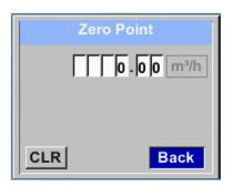
When, without flow, the installed sensor shows already a flow value of > 0 m<sup>3</sup>/h herewith the zero point of the characteristic could be reset.
