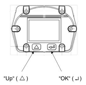
The operation of the VA 520 is done by the two capacitive key buttons Up  $(\triangle)$  and Enter (4)
