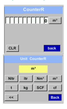
In order to change, e.g. the unit, first select by pressing key  $\_\Delta$  "the button "Unit" and then key "OK".
