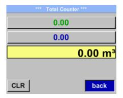
For changing one or both counter please select by pressing key " $\triangle$ " the corresponding counter-button then confirm it with key "OK".
