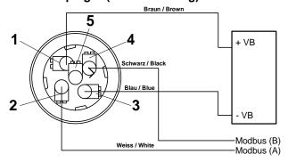
**Remark:** If the sensor is placed at the end of the Modbus system a termination is required. The sensors have an internal switchable termination, therefore the 6 fastening screws from the lid are to be released and set the internal DIP Switch to "On". It must be ensured that the connection plugs are still plugged and the gasket is installed correctly.
