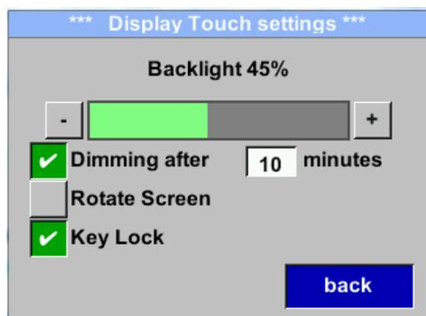
By activation of „**Key Lock**“ the operation of the sensor locked.
