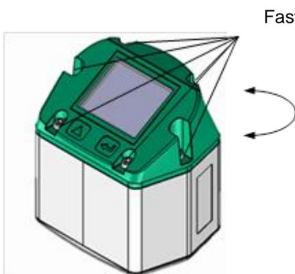
The Position of the Display head is twistable by 180° e.g. in case of reverse flow direction. For this purpose the 6 fastening screws are to be released and the display head rotated 180°.
