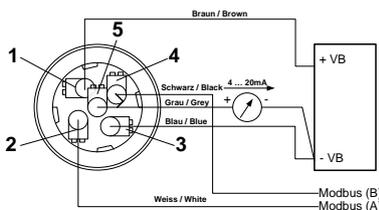
**Connector plug B (M12 - A-coding)**
