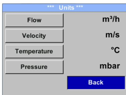
To make changes to the unit for the respective measurement value, first select by pressing „Δ“ the field of the „measurement value“ and activate „it with **„OK”** .
