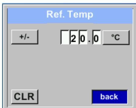
By pressing „Δ“ the position value is incremented by 1. Complete with **“OK”** and activate next number position.
