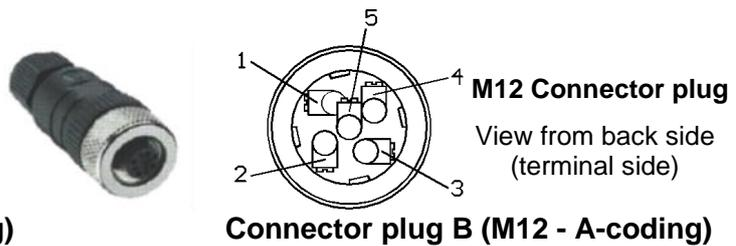
**Connector plug A (M12 - A-coding)**
