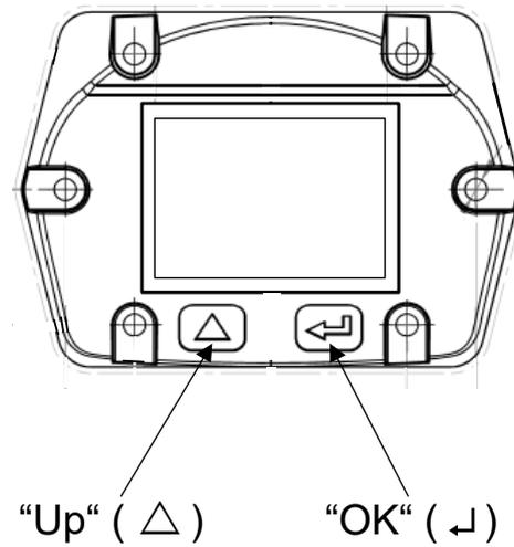
The operation of the VD 500 is done by the two capacitive key buttons Up (Δ) und Enter (←)
