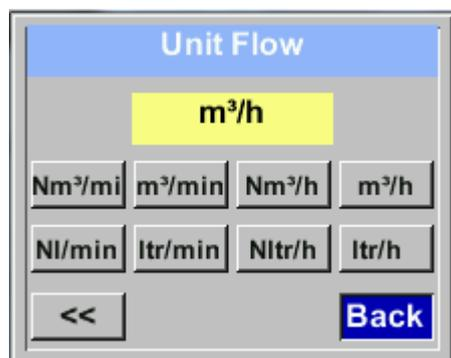
To the selected measurement value a corresponding / appropriate unit needs to be defined. Select „Unit“ with „ $\Delta$ “ and open menu with „OK“.
