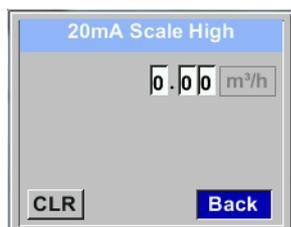
The scaling of the 4-20mA channel can be done automatically "Auto Range = on" or manual "AutoRange = off" .
