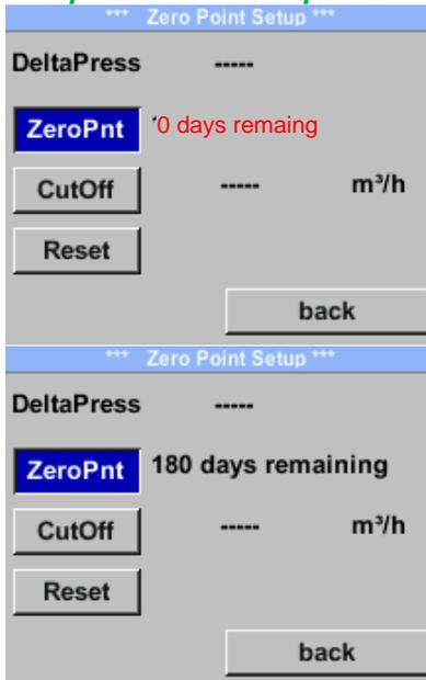
If the sensor shows the message **CalZeroPnt** in the display, then a zero point calibration should be carried out, see also chapter **Commissioning**.
