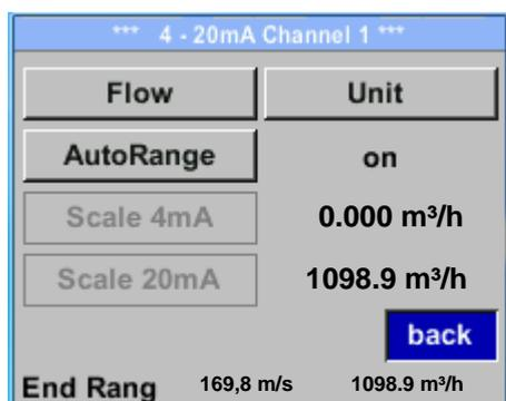
The 4-20 mA Analogue output of the Sensor VD 500 can be individually adjusted.
