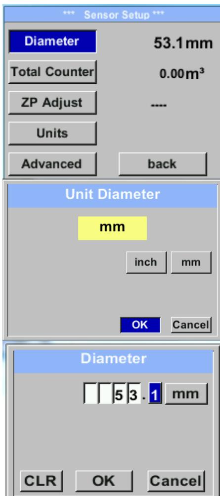
In order to change, e.g. the unit, first select by pressing key „ $\Delta$ “ the field **“Units”** and then key **“OK”**.
