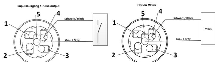
**Remark:** If the sensor is placed at the end of the Modbus system a termination is required. The sensors have an internal switchable termination, therefore the 6 fastening screws from the lid are to be released and set the internal DIP Switch to "On". It must be ensured that the connection plugs are still plugged and the gasket is installed correctly.
