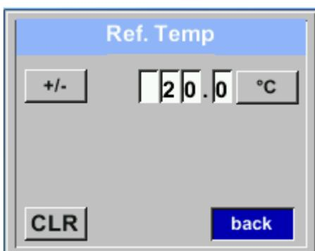
By pressing „Δ“ the position value is incremented by 1. Complete with “OK” and activate next number position.
