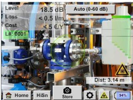
To use the measured distance for cost quantification, "Distance by laser" must be activated under "Parameters".
