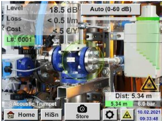
"Dist:" is green, the distance module measurement is robust, and the distance used is in the valid range.
