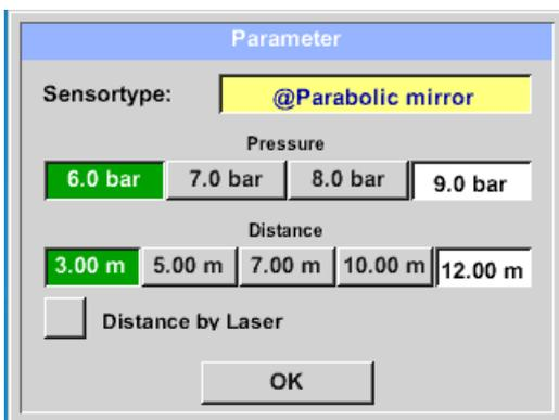
Note: Before "Distance by laser" can be activated, the laser must be switched on. Otherwise, the symbol flashes yellow and red.
