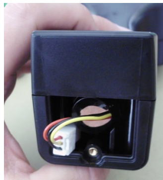
Disconnecting the connector
