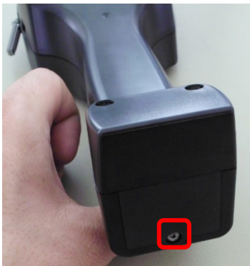
Removing the battery cover
