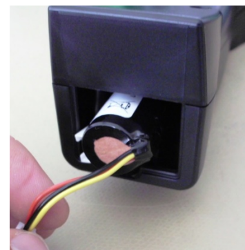
Carefully pull out the battery
