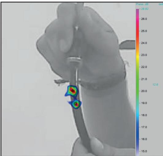
With the “acoustic zoom” of the LeakCam 600, leaks can be precisely localized from far distances by focusing ultrasonic noises even more strongly. In combination with the optical zoom (x2, x4, x8), this gives you a clear visual magnification of the inspected components. This allows you to detect leaks quickly and accurately - even in areas that are difficult to access
