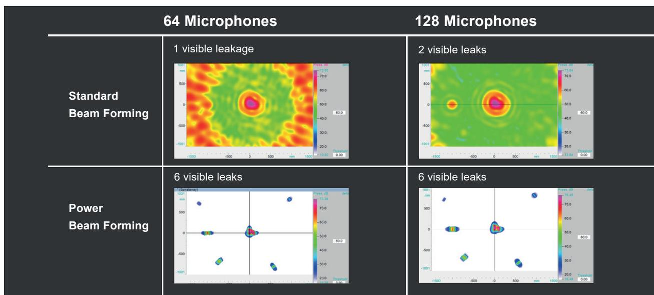
Thanks to the Power Beam Forming process and the associated dynamics, the LC 600 can fully exploit the advantage of the large image aperture angle. The device can check an area of 4 x 3m from a distance of 3m at a glance - without missing any small leaks.
