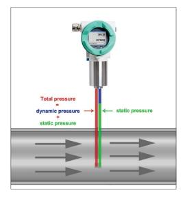
The integrated, precise differential pressure sensor measures the differential pressure/ dynamic pressure at the sensor tip. The pressure depends on the respective gas velocity. The flow is therefore easy to determine by means of the pipe diameter.
