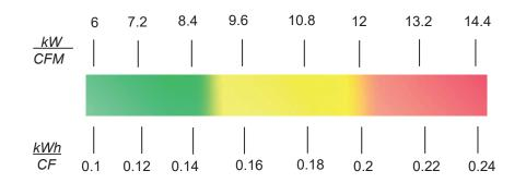
Typical specific power requirement for an oil-injected compressor
