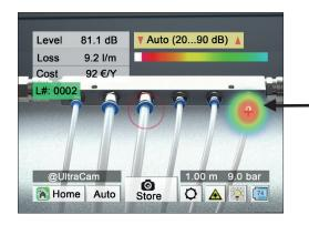
The UltraCam LD 500 / LD 510 uses 30 MEMS microphones to calculate and visualise the ultrasound image. In addition, the device makes inaudible ultrasound audible
