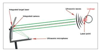
By focusing the ultrasonic waves in the parabolic mirror, even the smallest leaks of 0.8 l/min (approx. \$8 annually) can be located with pinpoint precision (± 6 in.) at a distance of 32 to 50 ft.
