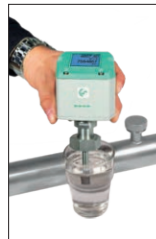
The sensor can be removed and cleaned
