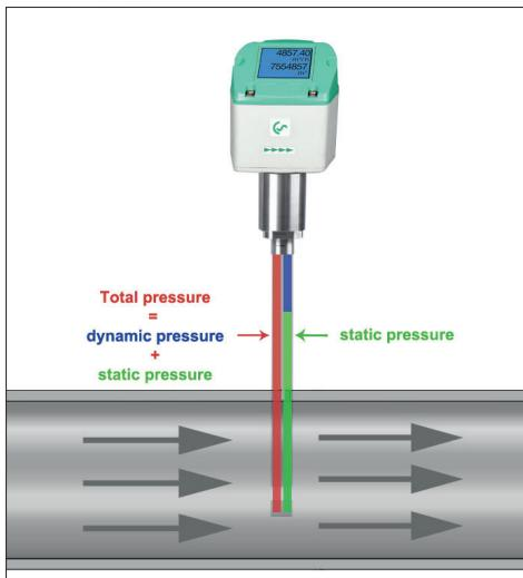
The integrated, precise differential pressure sensor measures the differential pressure/dynamic pressure at the sensor tip. The pressure depends on the respective gas velocity. The flow is therefore easy to determine via the pipe diameter.
