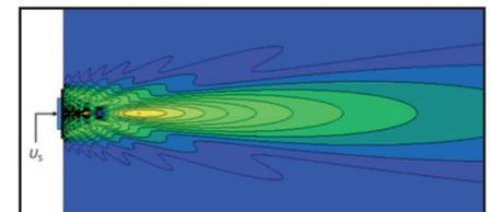
**Fig. 12: Ultrasonic field of a spherical source**
