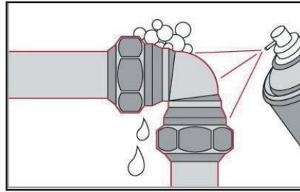
**Fig. 14: Functionality of the Leak Detection Spray**
