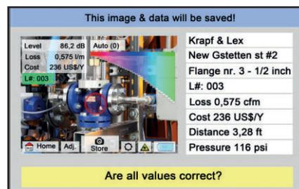
The stored data can be exported to any commercially available USB stick and evaluated with the optionally available PC evaluation software "CS Leak Reporter".
