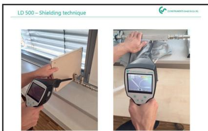
Compressed air leaks generate a strong ultrasonic field, which can possibly generate an ultrasonic signal in the entire room.
