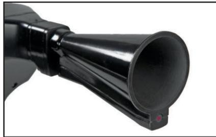
The acoustic trumpet bundles the sound waves of small compressed air leaks and thereby amplifies the audible signal. At the same time, it prevents lateral sound waves from hitting the ultrasonic transducer, making it easier for the user to locate the leakage.
