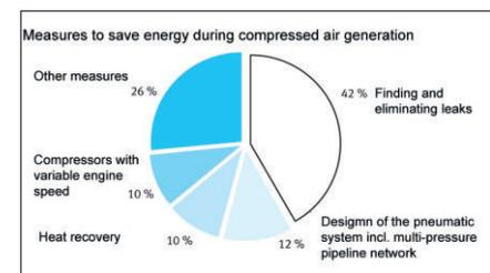
**Fig. 5: Savings potential of a compressed air system**
