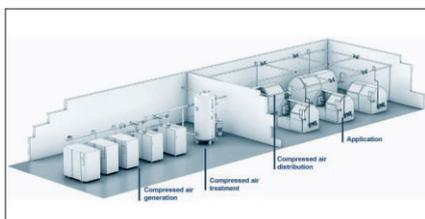
**Fig. 1 Components of a compressed air system**
