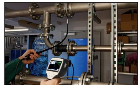
Since some compressed air lines are difficult to access, a flexible gooseneck can be used. This serves as an extension of the arm for leaks that are far away and difficult to access.
