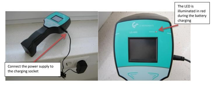
The LD400 checks the charge status of the battery and automatically starts the charging process. The following scenarios are possible:
