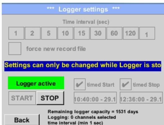
The data logger can be started without activated time settings, use the *Start* and *Stop* buttons for activate and disable.
