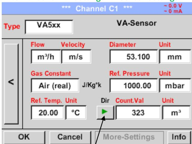
In case of a bidirectional sensor (VA5xxB) can be changed here by pressing the key to switches the other direction and thus the second counter reading is entered
