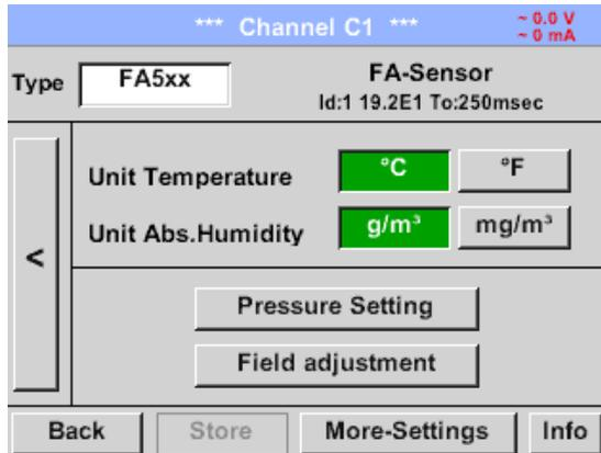
Unit selection for temperature and humidity by pressing the button °C, °F, g/m<sup>3</sup> or mg/m<sup>3</sup>.
