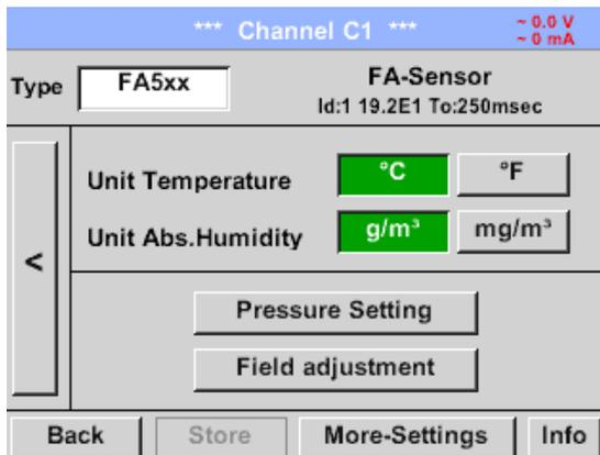
The system pressure is inserted by entering the values in the corresponding text field. The unit can be freely selected, selection menu is opened by pressing the corresponding button units
