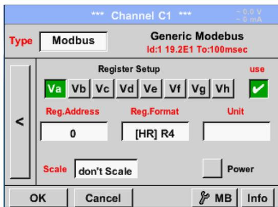
Via Modbus, it is possible to read out up to 8 Register-Values (from Input or Holding Register) of the sensor.
