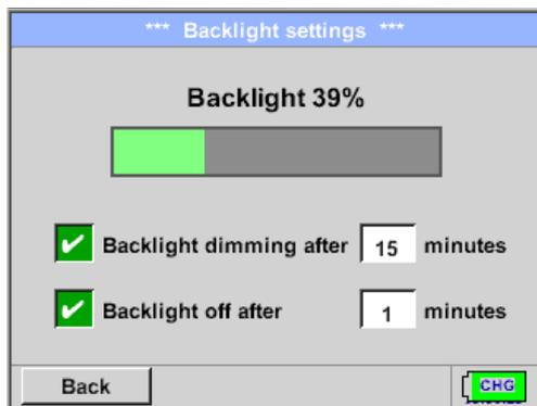
To reduce the energy consumption (device runtime), you can switch off the display backlight by setting "*Backlight off after*".
