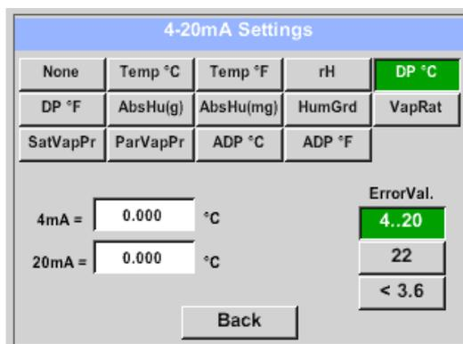
This menu allows the adjustment / assignment of the measurement value and the scaling of the analogue output.
