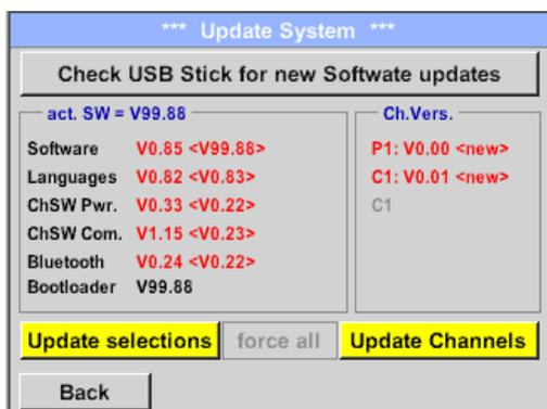
If the LD 500 is correctly connected to the USB stick and there are new versions of the individual SW Parts, the new versions are marked in red.
