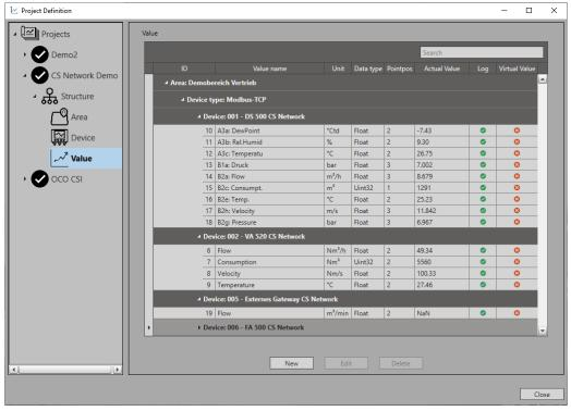
After this step, the configuration of the devices and measured values is completed. The program is restarted.
