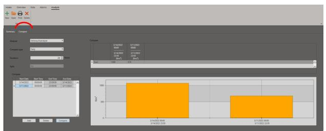
Then select the corresponding analysis, the comparison type and the duration. After that, use the "Add" button to define the comparison periods. Use the "Compare" button to start the comparison and the corresponding diagrams and statistics tables will appear.
