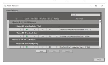
First select under "Alarm type" the condition that should apply and then under "Threshold", the threshold value when the alarm is triggered. You can also set a delay that determines how long the threshold value must be violated before the alarm goes on (tOn) or off (tOff). Next, assign the alarm to the corresponding measured value under the "Show values" button and a predefined text will appear in the "Alarm text" field. You can edit this text by using the checkbox "User defined text".
