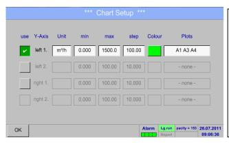
The *Plots* description field shows on what channel the measured data were recorded and there can be seen how much recordings on one y-axis are represented.
