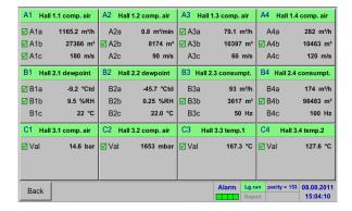
The overview of *Real time values* shows the current measured values of all connected sensors.
