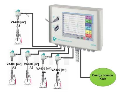
Calculated are the complete consumption of air and energy as well as the "specific performance" of the entire system.
