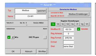
The *Modbus ID* is at initial activation taken over as a copy of the *Modbus settings* of the base channel (marking: value in <>), but it can be overridden.
