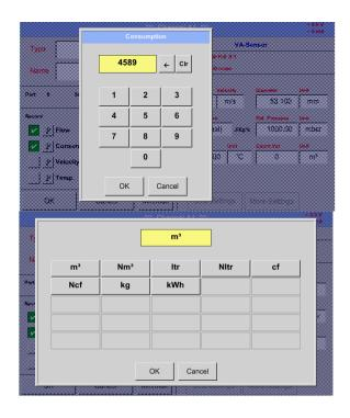
The sensor allows taking over a starting counter value. Inserting the value by entering the "Count. Val." text field.
