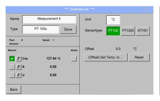
Here the sensor type *PT100* and the *Unit* in °C are chosen, alternatively the sensor types *PT1000* and *KTY81*, as well as the Unit °F can be selected.
