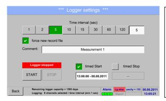
By pushing the *timed Start* button and then the date/time description field below, the date and the start time can be set for a data logger recording.
