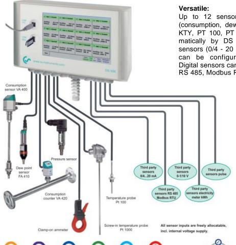
Up to 12 sensors, incl. all CS sensors (consumption, dew point, pressure, current, KTY, PT 100, PT 1000) are identified automatically by DS 500. Optional analogue sensors (0/4 - 20 mA, 0 - 1/10/30 V, pulse) can be configured easily and quickly. Digital sensors can be connected via RS 485, Modbus RTU and SDI.
