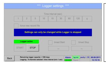
The data logger can be started without activated time settings, use the *Start* and *Stop* buttons for activate and disable. Left below there will be shown how many values are recorded and how long there still can be recorded.
