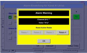
By activated R*elais* button, it is allowed / possible to turn off the corresponding alarm relays in the popup appearing in alarm case.
