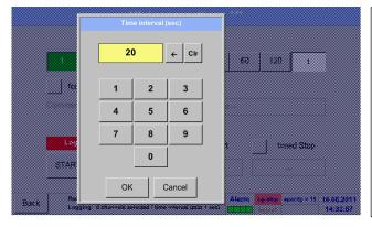
A different, individual *Time interval* can be entered in the highlighted white description field right at the head, where the currently set *Time interval* is always displayed.
