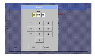
By changing the text field values the new delay time could be defined. Here for *Delay T1*.
