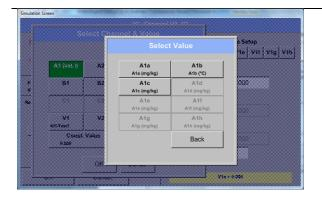
Pressing the respective channel button e.g. *A1b* will select the measurement channel
