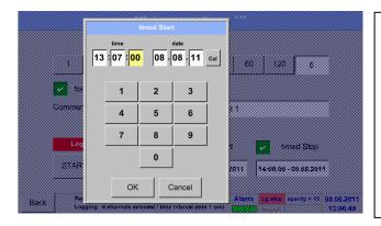
After pushing the *date/time description field* a window will appear where the yellow marked area of the time or date can always be set and changed.
