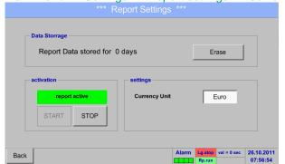
By pushing of the *Currency Unit* description field, a currency may be entered, which is applied to the **Consumption report** and the **cost settings**.
