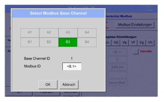
The *Modbus ID* can be taken from a base channel (inherited). This inheritance allows a change in the base channel simultaneous acquisition of change also for the extended channel.
