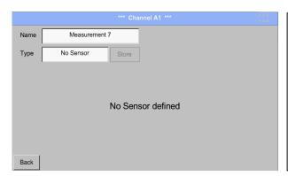
Is used to declare a not currently needed channel as *No Sensor defined*.
