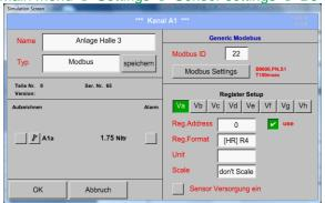
Via Modbus it is possible to read out up to 8 Register-Values (from Input or Holding Register) of the sensor.
