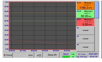
If there is no grid entered in the setup, *min* will be 0, *max* 100 and *step* 10 (Setup #3).
