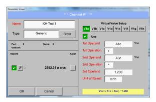
Use the *Record* buttons to select the measurement data that will be stored by **activated data logger**.
