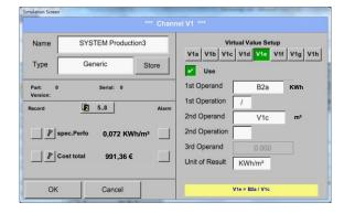
Calculation of the *specific. Perfor.* Is done in V1e with V1e = B2 / V1cFor this example, it is 0,072 KWh/m<sup>3</sup>
