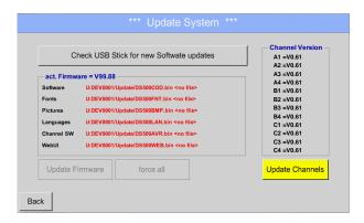
If after pressing the button "Check USB Stick for new Software updates" the following messages appear in the window, is the DS 500 is not properly connected to the USB flash drive or there are no files available.
