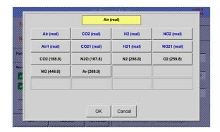
All gases marked in blue and with (real) have been a real gas calibration curve stored in the sensor.
