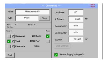
Typically the value with unit of **1 Pulse** is standing on the sensor and can directly entered to the **1 Pulse** = description field.
