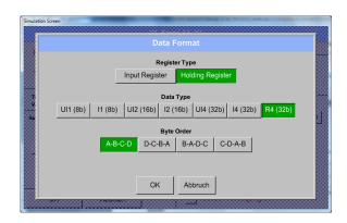
With the buttons *Input Register* and *Holding Register* the corresponding Modbusregister type will be selected.
