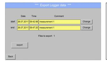
Use the *Change* buttons to adjust a period between *start* and *end*. Stored measurement data in this period are exported.
