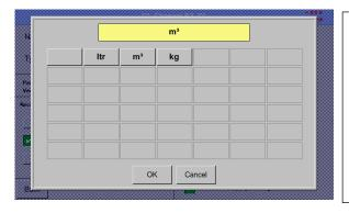
The available Units for the Unit of Counter by *Type* **Pulse**
