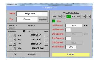
For a complementation, we added in *V1d* the total sum of consumed energy. Read out of electric meter at input B2.
