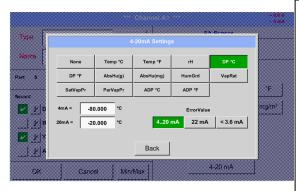
This menu allows the adjustment / assignment of the measurement value and the scaling of the analogue output.
