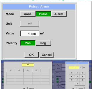
To set up the pulse first the unit and the measurement value have to be defined.
