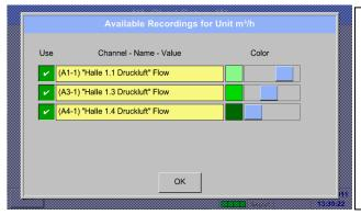
5. Several recordings with the same unit can be represented in one y-axis, with the help of various colour intensities.
