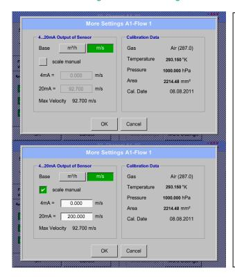
In *More-Settings*, you can define whether the 4 - 20 mA analogue output of the sensor based on the flow rate or velocity.
