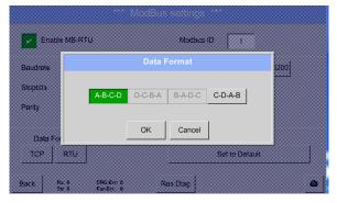
For using the DS 500 as RS485 Slave, first it is requested to enable it by activation of of *Enable Modbus RTU(RS485)*.
