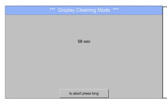
This function can be used for cleaning the touch panel during running measurements.
