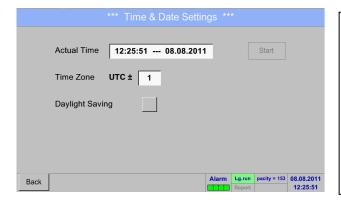
By pushing the *Time Zone* description field and enter the correct *UTC*, you can set the correct time all over the world.
