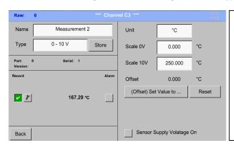
Please see the scale of the sensor (here for example Type  $\bf 0$  -  $\bf 10V$  corresponds to  $\bf 0$  -  $\bf 250\,^\circ$  C) from the data sheet of the connected sensor.
