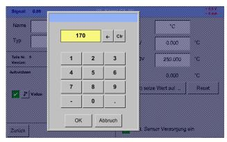
With *Set-Value to-(Offset)* it is possible to set the measurement data to specific value.
