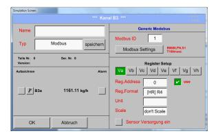
The measurement values are kept in the registers of the sensor and can be addressed via Modbus and read by the DS500.
