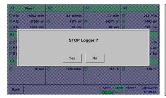
If the data logger is activated, the following window will appear and via pushing Yes it can be disabled.
