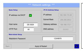
Here you can set up and made a connection, with or without *DHCP*, to a computer.
