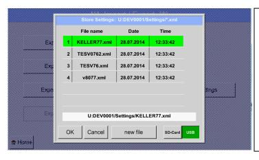
With Export system settings, all existing sensor settings can be exported to a USB stick or to the internal SD card. It stores all sensor settings including recording-, alarm-, graphics-, value-and name definitions.
