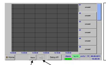
One or more channels for the recording and presentation of measured data can be selected here, such as a dew point sensor or several different sensors.
