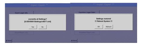
After confirmation with OK it is asked again if settings should be overwritten, by confirming this once more the new System Settings are loaded and a reboot is required.
