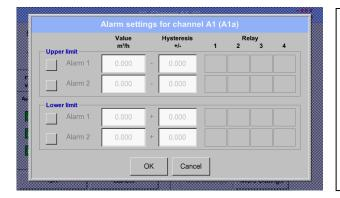
In the alarm settings, an *Alarm 1* and *Alarm 2* incl. *Hysteresis* can be entered for each channel.
