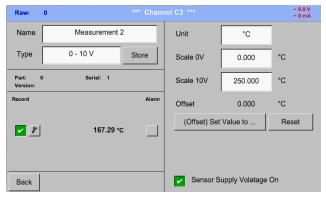
The Sensor Supply Voltage is switched On, if it's required by the sensor type, otherwise off (no green hook).
