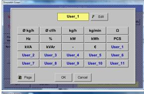
By pressing the button *Edit* you enter the menu for inserting the new Unit.
