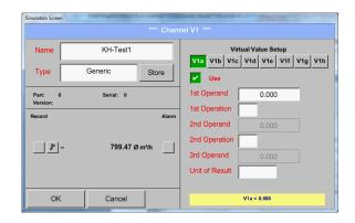
Every virtual value has to activated by selecting the respective *Value-Button* e.g. *V1a* and pushing of the *Use Button*.
