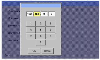
After pushing, for example the *IP address* description field, the command window appears, where in the selected yellow area a partial *IP address* can be entered manually.
