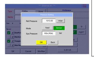
By using an ext. pressure sensor, which is detected automatically e.g. here at input B1, the button *Sensor* has to be activated.
