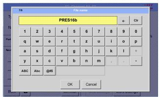
In case of a new file, by pressing the *new file* button, the chosen name must be entered and confirmed with *OK*.
