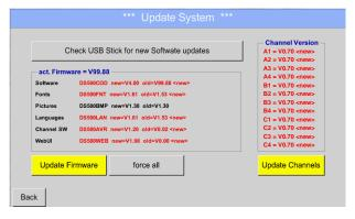
Is the DS 500 properly connected to the USB drive and there are new versions of the individual software parts available, then they are in red font and <new> marked.
