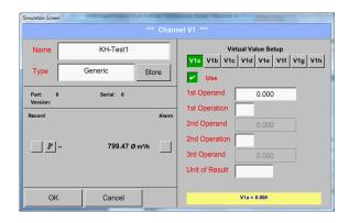
By accessing the text field 1st Operand The list with all channels (HW and virtual channels) and const. Value appears.
