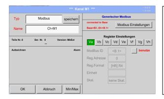
Via Modbus, it is possible to read out up to 8 Register-Values (from Input or Holding Register) of the sensor.
