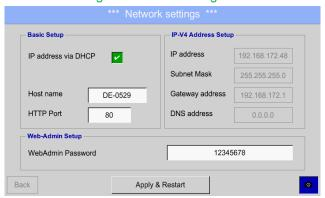
In the text description field *WebAdmin*Password could the password be set up.
