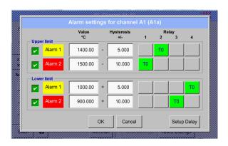
E.g. set the *Alarm 1* to relay 2 and relay 4 and the *Alarm 2* to relay 1 and relay 3.
