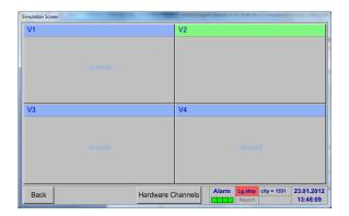
After pushing the button "*Virtual Channels*" in the Sensor Settings menu an overview with the 4 available "*Virtual Channels*" is displayed.
