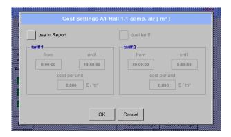
In the *Sensor settings* for the *Type* **CS-Digital** and **Pulse** you can enter the costs per unit in the *Cost Settings*.
