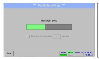
Here you adjust the desired *Backlight* (15-100%) of the display directly.
