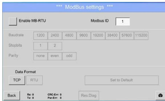
Enable the RTU Modbus by activation of the "**Enable MB-RTU**" button.
