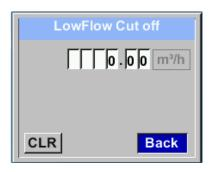
With the low-flow cut off activated, the flow below the defined "LowFlow Cut off" value will be displayed as 0 m³/h and not added to the consumption counter.
