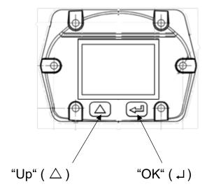
The operation of the VA 521 is done by the two capacitive key buttons Up ( $\triangle$ ) and Enter ( $\downarrow$ )
