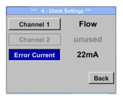
This determines the output in case of an error at the analog output.
