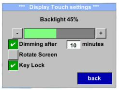
With the button "-" and with button "+" it is possible to adjust the backlight / display brightness. The actual / adjusted backlight brightness is showed in the graph "Backlight."
