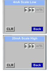
The scaling of the 4-20mA channel can be done automatically "Auto Range = on" or manual "AutoRange = off".
