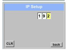
For manual (static) IP, the "IP Address", "Subnet" and "Gateway" selection keys must be selected and activated with "OK".
