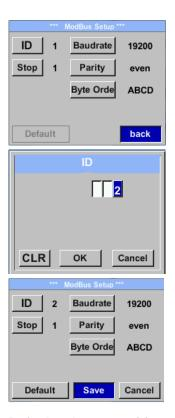
For changes, e.g. the sensor ID, first select by pressing key  $\_\Delta$ " the field "ID" and then key "OK".
