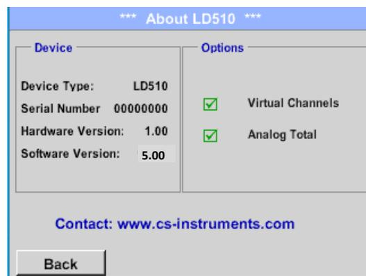
In the example the hardware version is 1.00 and therefore not intelligent. → In this case, CS INSTRUMENTS can replace the mainboard.
