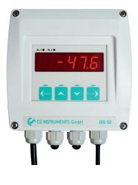
The DS 52 has 2 potential-free alarm contacts (changeover contacts) which can be charged with a maximum of 230 VAC, 3 A. The alarm thresholds are freely adjustable with the keys. The display is supplied with 230 VAC and has an internal mains unit which provides a voltage of 24 VDC/100 mA for the sensor.
