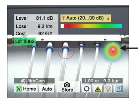
The UltraCam LD 500/510 uses 30 MEMS microphones to calculate and visualise the ultrasound image. In addition, the device makes inaudible ultrasound audible
