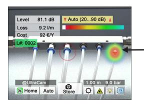
The UltraCam LD 500/510 uses 30 MEMS microphones to calculate and visualise the ultrasound image. In addition, the device makes inaudible ultrasound audible
