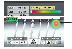
The UltraCam LD 500/510 uses 30 MEMS microphones to calculate and visualise the ultrasound image. In addition, the device makes inaudible ultrasound audible
