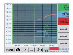
So the user can take a look at the stored measurement curves also without any computer at any time on site. This grants a quick and easy analysis of the compressed air or gas consumption.
