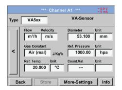
Threshold value exceedance can be reported optically and acoustically. 2 relays for pre- and main alarm are freely adjustable.
